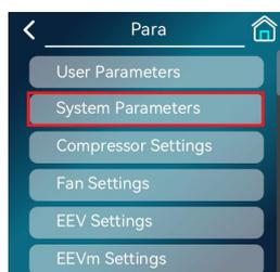
Click “System parameters” option, then scroll down and click “Smart grid” to turn “ON” or “OFF” the function.
