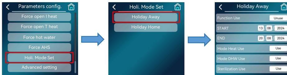
Application example: Assuming that it is now January 3, 2020 and you will be going out for a fortnight in three days, which means going out on January 6, 2020 and coming home on January 20, 2020. You can set up the function as shown in the table below in order to prevent the waterways from freezing.
