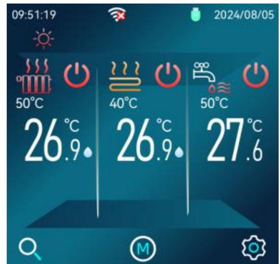
The system includes dual zone air conditioning control (Zone A + Zone B) and domestic hot water control.
