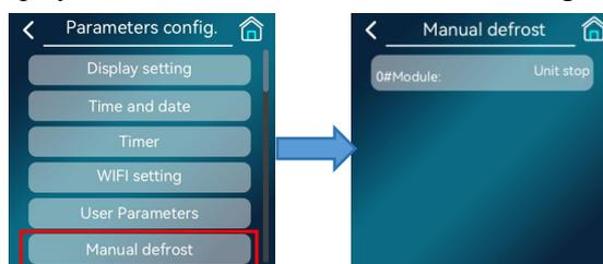
Only when the module is in the operation, the water temperature, fin temperature and other conditions are met, can the defrosting be successfully entered by clicking the corresponding item. At this time, the current state of the module will be switched to defrosting. Otherwise, it will maintain the original status.
