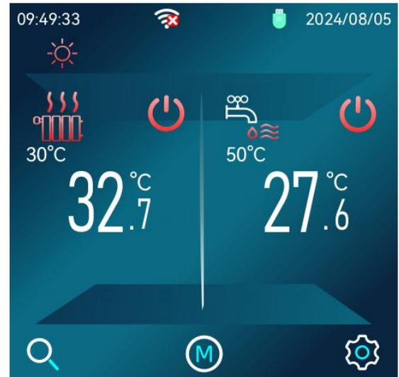
The system includes single-Zone Air conditioning room temperature control and domestic hot water control.
