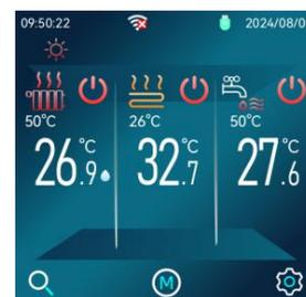
8.6.5 Two-zone water temperature + Hot water: The system includes two-zone air conditioning water temperature control (Zone A can be heated or cooled, and Zone B can only be heated) and domestic hot water control.
