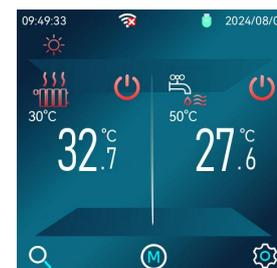
8.6.4 Two-zone mixing + Hot water: The system includes two-zone air conditioning water temperature (Zone A) + room temperature (Zone B) control (Zone A can be heated or cooled, and Zone B can only be heated) and domestic hot water control.
