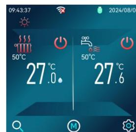
8.6.3 Single-zone room temperature + Hot water: The system includes single-zone air conditioning room temperature control and domestic hot water control.
