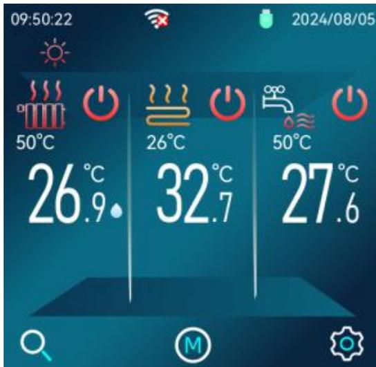
The system includes dual zone air conditioning control (Zone A water temperature + Zone B room temperature) and domestic hot water control.
